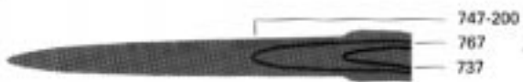
The diagram above indicates that a 767, 737 and similar aircraft leave a significantly smaller imprint than 747-200 series aircraft
